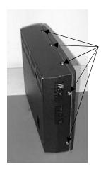
Holes for retaining screws
