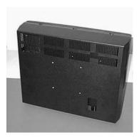
5. Fasten the cover to the monitor with the 7 retaining screws included in the installation kit. Three screws will fasten across the top of the cover and two on each side, as shown in the illustration on the next page.
