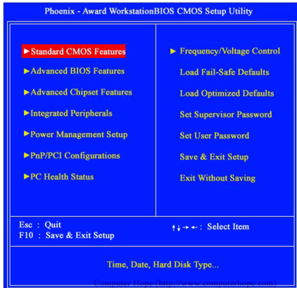
Figure 3-6: The Phoenix - Award CMOS Setup Utility Main Menu
