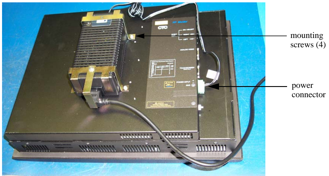
Figure 2-2: Mounting an External AC Adapter
