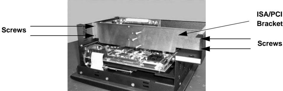
3. Remove the card tang of the slot in which you intend to place the card.:
