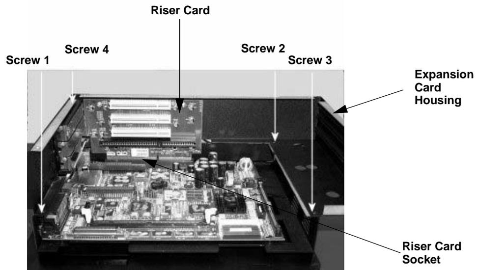
2. Attach the new expansion card housing using the 4 screws included in the kit. You can only access Screw 4 through the opening at the edge of the expansion housing as shown above.
