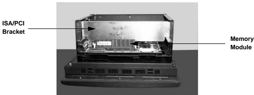
8. Remove the bracket that holds the ISA/PCI bracket (shown above) and any ISA or PCI cards you have installed.
