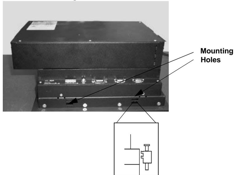
2. Attach the mounting clamp(s) on the elongated side.
