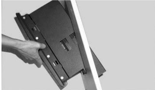
3. If the back cover is still removed, continue to the next step. If you replaced the back cover, remove it by removing the 5 screws that hold the cover in place.
